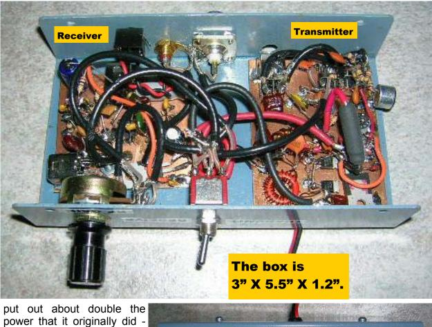
power that it originally did about 2 watts. I found that the regulator also needed a bypass capacitor to keep the RF off of the output or there was some instability.
