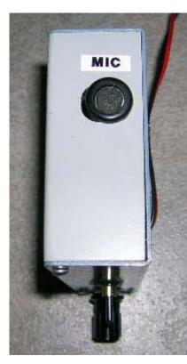
The transmitter has been tested underground. Using a similar power level with the Yaesu FT-817ND has shown that effective communications can be done at least as deep as 220 feet below the surface in dry limestone. I was very pleased. See the article on Grand Canyon Caverns underground radio.
