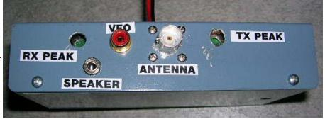
some time ago and seemed perfect for this project. It is housed in a separate metal box (the seemingly ever present mint tin) for shielding. The external VFO can also be changed to a crystal controlled oscillator, a different type of VFO (maybe digital controlled), or maybe a PTO (permeability tuned Oscillator). With so many options, it made sense to use an external frequency source.
