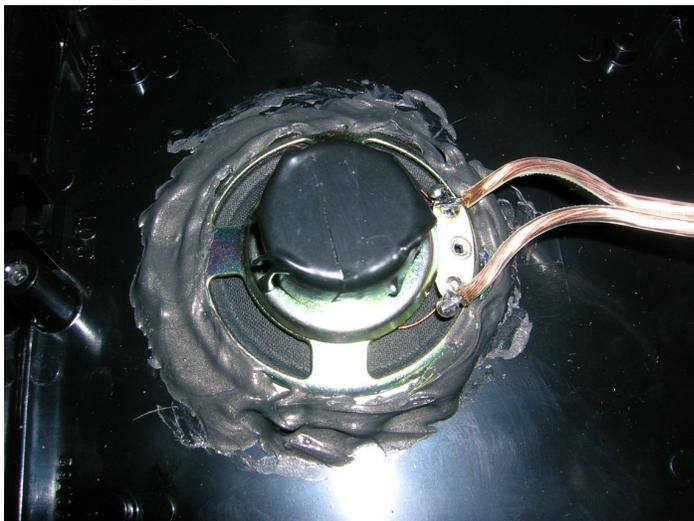
The speaker was mounted onto the case with a generous amount of automotive silicone. I prefer the Ultra Black variety of silicone since it cures rapidly and has strong adhesion.
