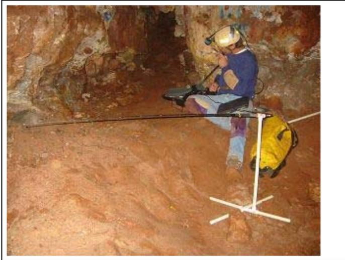
With the success of other reported HF radio use underground (most recently by Bonnie Crystal in SPELEONICS 24), some experiments were undertaken to see what was possible at 80 meters in the US ham bands using commercial off the shelf equipment. Both voice and data, using PSK31, were tried with success. Various antennas were tried with varying rates of success.
