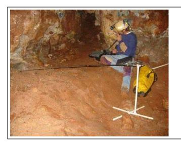
With the success of other reported HF radio use underground (most recently by Bonnie Crystal in SPELEONICS 24), some experiments were undertaken to see what was possible at 80 meters in the US ham bands using commercial off the shelf equipment. Both voice and data, using PSK31, were tried with success. Various antennas were tried with varying rates of success.
